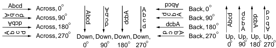
Figure 50. 3816 Inline Directions and Character Rotations for Downloaded Fonts
